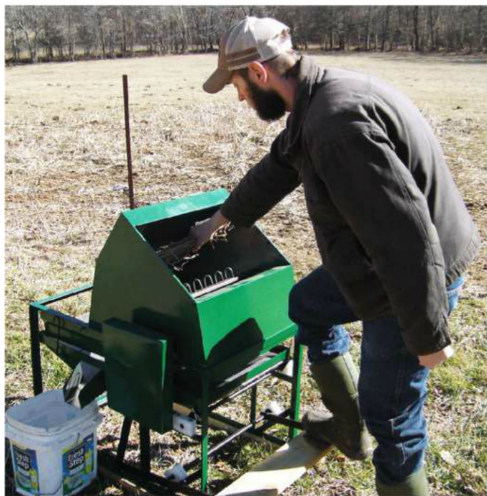
A treadle-powered thresher, such as this one from the Back to the Land Store , can speed up processing. See a video of one in action at http://goo.gl/hJNdqk .
